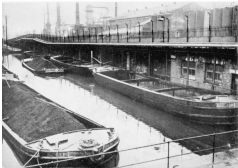
N.C.B. boats in the basin at Barton. The assortment (all dumb boats) includes short and long craft, and round and transom sterns. Courtesy: The Guardian
