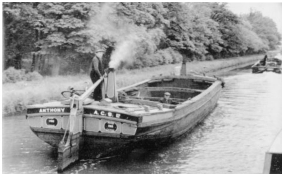
Square-transomed "Anthony" is towed past Scarisbrick by "Nidd." "Anthony" displays many of the features of Yorkshire Craft, including square chimney, and was brought over the Pennines from Airedale Canal Services. Courtesy: J. Parkinson
